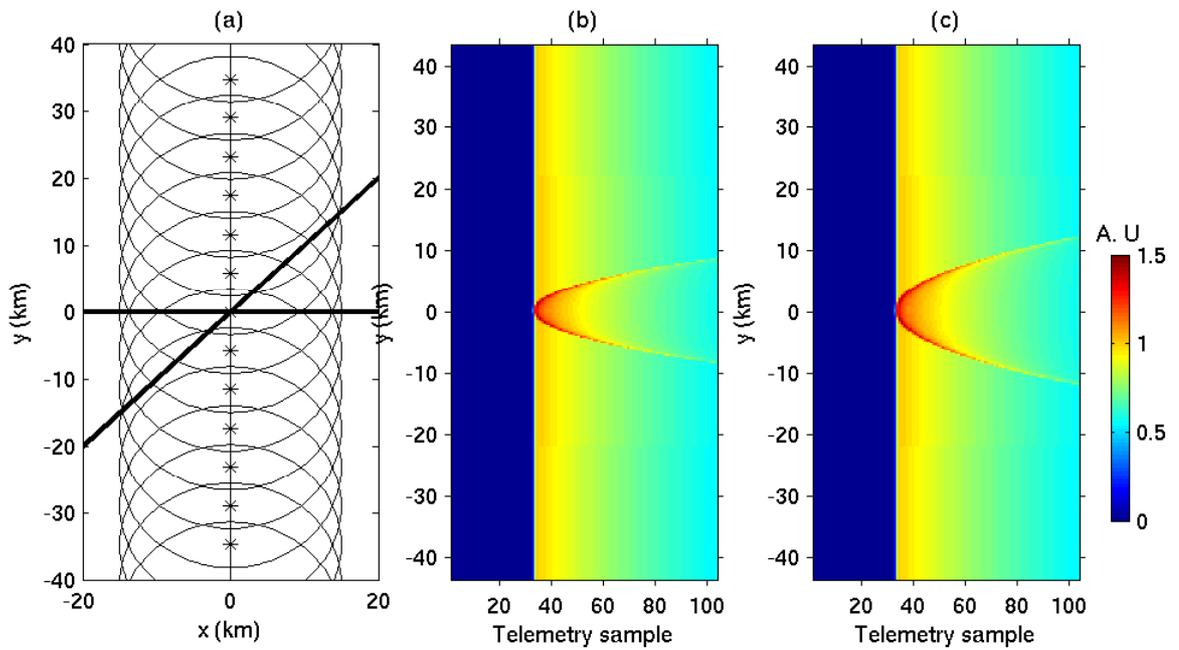
**Figure 4.** Jason altimeter echo waveforms in presence of simple surface slicks of 10 dB relative brightness and 100 m width. [a] schematic diagram showing the slicks (heavy solid lines) and the altimeter footprint (circles, 1 per second). Modeled waveforms for perpendicular slick (b) and the 45° oblique slick (c). The waveform colorscale is in arbitrary units (1 correspond to the maximum value of the Brown model).
