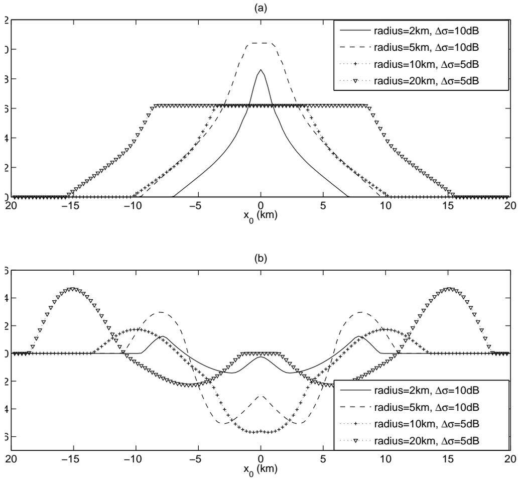
**Figure 9.** Variation of  $\sigma_0$  induced by the slick for different radii and relative brightness, (b) of off nadir angle estimates.
