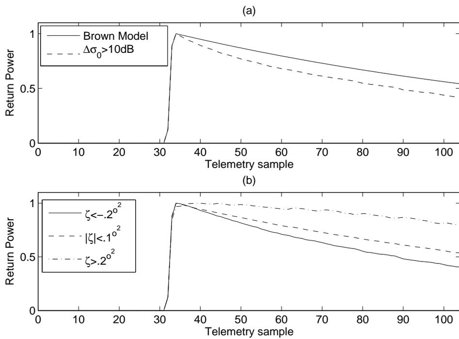
**Figure 12.** Mean normalized altimeter waveforms of Figure 11, sorted according to  $\sigma_0$  (a), and sorted according to off-nadir angle (b).
