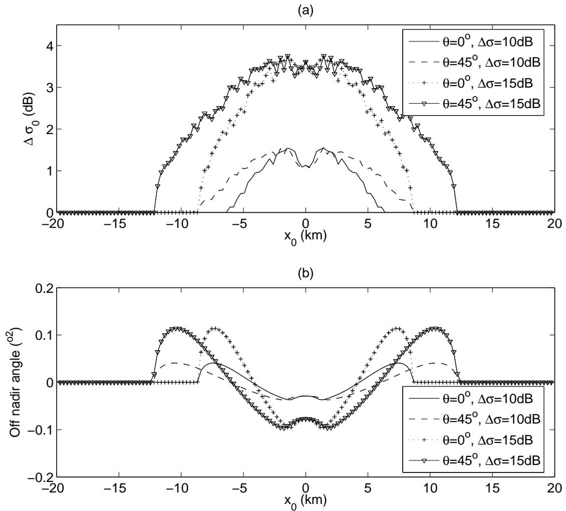
**Figure 6.** Variation of  $\sigma_0$  induced by the linear slick for different angles and relative brightness, (b) variation of off nadir angle estimates.
