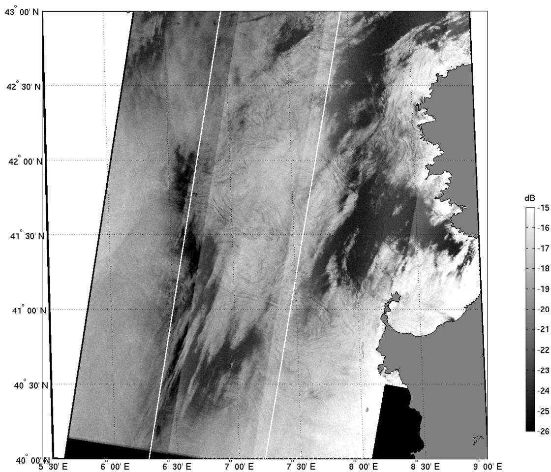
**Figure 1.** Radarsat Image taken on April 24 2004 off the coast of Corsica under low wind speed conditions (less than 1.5 m/s) showing zone of little backscatter (dark patches) and slick like features.
