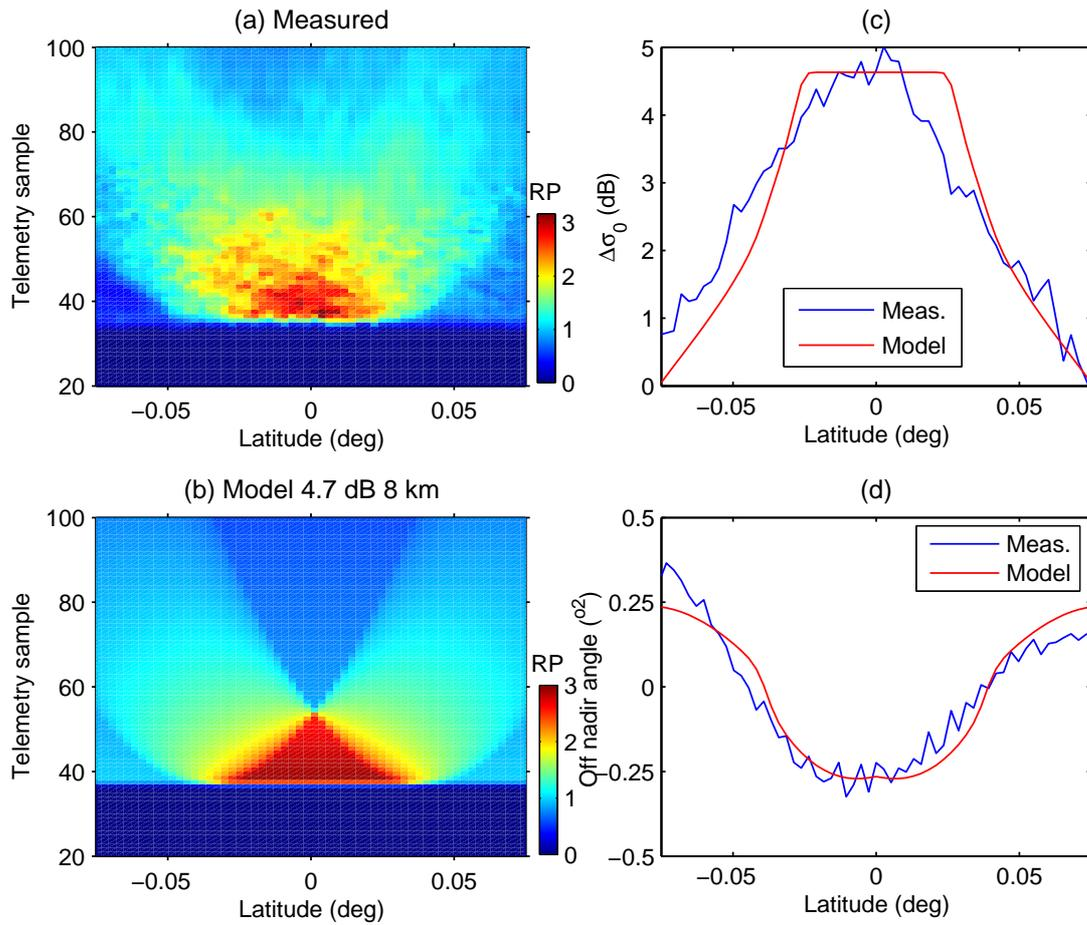
**Figure 13.** Best fit of observed waveforms. Jason waveforms near  $1.4^\circ$  S for cycle 107 pass 14 (a), modeled waveforms for a 8 km, 4.7 dB relative brightness circular patch (b), observed and modeled relative  $\sigma_0$  variation (c), observed and modeled off nadir angle (d). The waveform colorscale (R.P. i.e. Return Power) is in arbitrary units.
