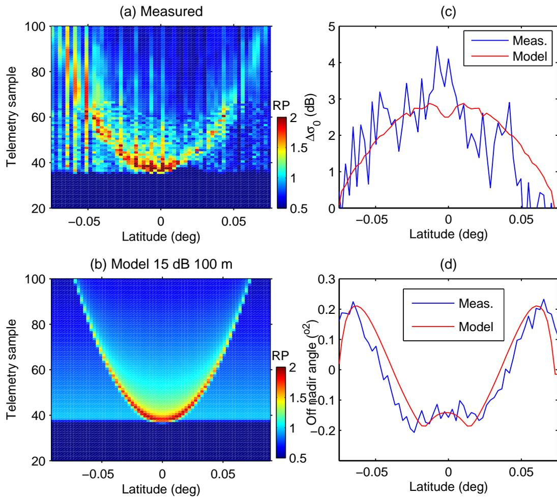
**Figure 14.** Best fit of observed waveforms. Jason waveforms near  $1.4^\circ$  S cycle 107 pass 34 (a), modeled waveforms for a 100 m, 15 dB relative brightness linear slick (b), observed and modeled relative  $\sigma_0$  variation (c), observed and modeled off nadir angle (d). The waveform colorscale is in arbitrary units.
