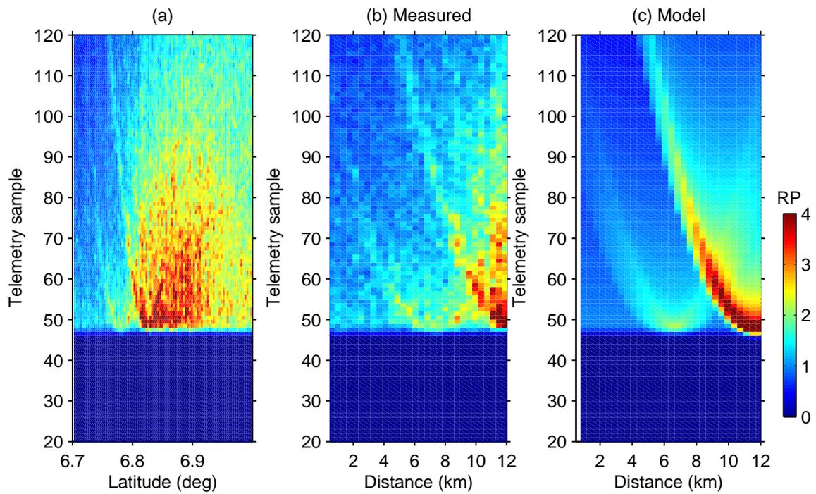
**Figure 15.** Best fit of observed waveforms, Envisat waveforms near  $6-7^{\circ}$  N for cycle 10 pass 94 (a), Details of the waveforms near  $6.7^{\circ}$  N showing the 2 V-shaped patterns (b), modeled waveforms (c). The waveform color scale is in arbitrary units.
