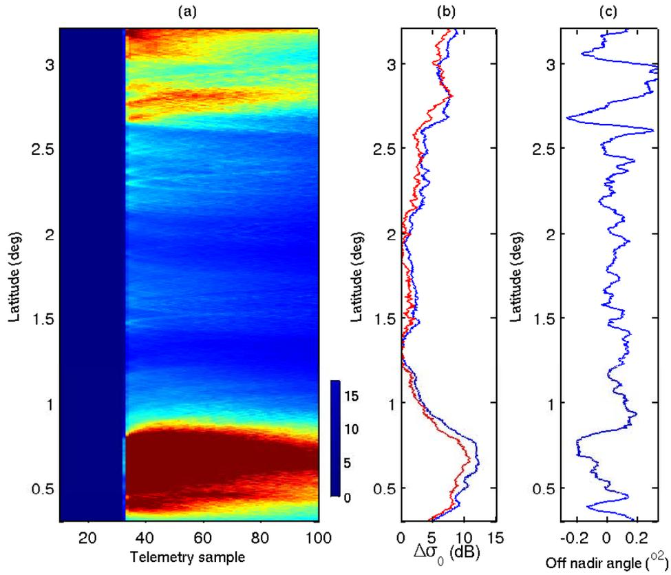
**Figure 11.** Modeled waveforms for a Jason type altimeter using the surface  $\sigma_0$  of Figure 10 the colorscale is in Arbitrary units (a). Relative variation of  $\sigma_0$  estimated from the waveforms (blue line) and mean surface  $\sigma_0$  over the altimeter footprint (b). Estimate of off nadir angle (c).
