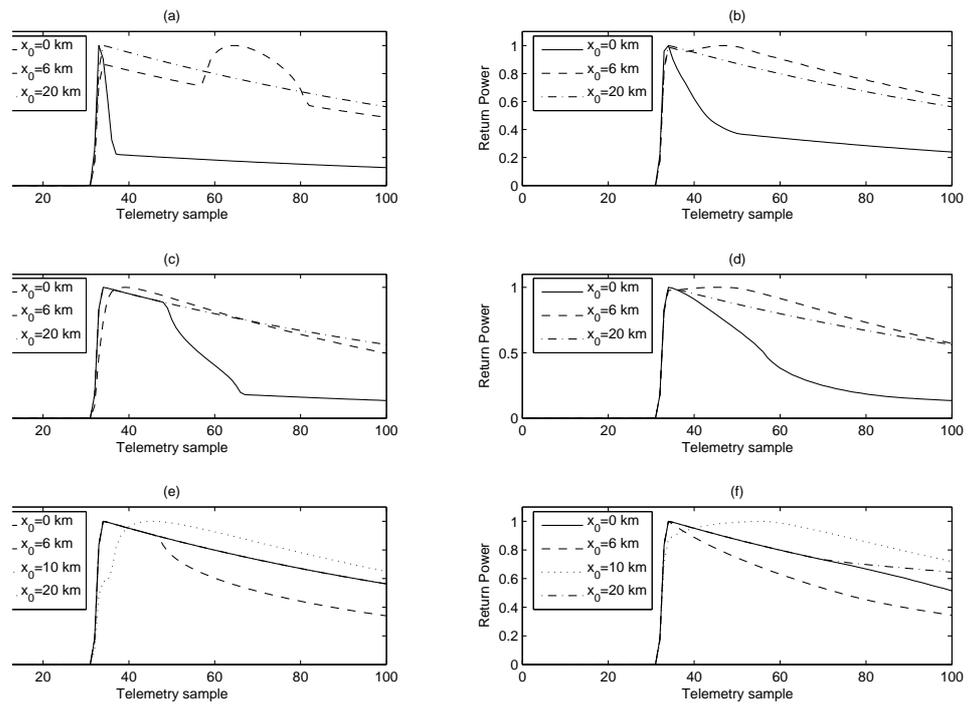
**Figure 8.** Jason altimeter normalized echo waveform in presence of circular surface slicks. High rate waveforms for different distances  $x_0$  between the satellite nadir and the slick (a), and 1-s average waveforms for the same  $x_0$  (b) for the 2 km radius 10 dB slick. Idem for a 10 km radius 5 dB slick (c) and (d). Idem for a 20 km radius 5 dB slick (e) and (f).
