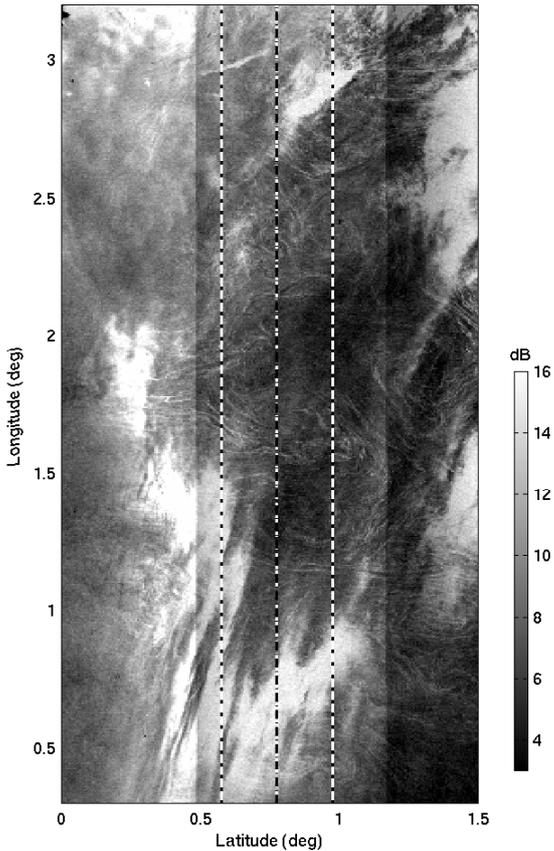
**Figure 10.** Surface  $\sigma_0$  in dB estimated from the Envisat SAR image of Figure 2. The dash-dotted line represent the altimeter ground track and the dotted line the altimeter footprint.
