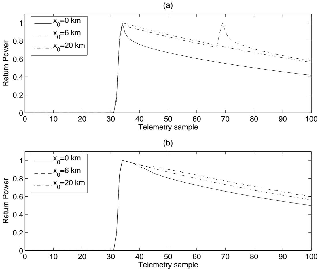
**Figure 5.** Jason altimeter normalized echo waveform in presence of a simple surface slick of 10 dB relative brightness and 100 m width. (a) High rate normalized waveforms for different distance  $x_0$  between the satellite nadir and the slick, (b) 1-s average normalized waveforms for the same  $x_0$ .
