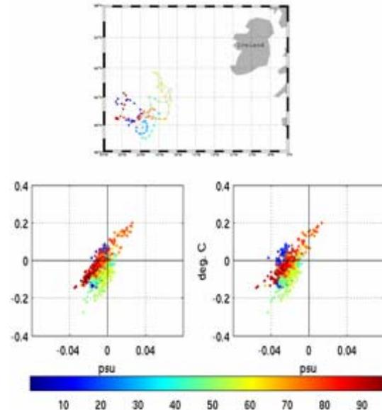
*Figure 1: Sensitivity test. Top: trajectory of the ARGO profiler used in the test. Bottom: diagram of the temperature and salinity residuals at 7000 m, left: unperturbed float, right: float perturbed with a constant -0.04 PSU offset.*
