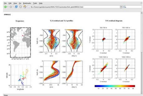
Figure 4: Graphic tools used for screening the ARGO profilers residuals over their lifetime.
