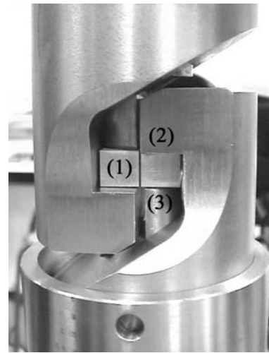
1 - small bonded sample 2 - support 3 - fastening device
