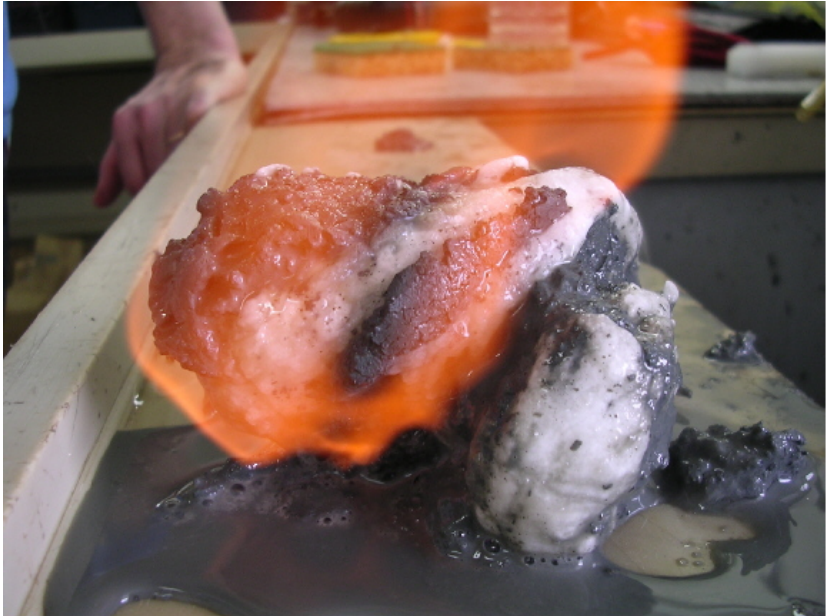
Photo 1 : Photography of solid sample of gas hydrate 10 cm diameter
