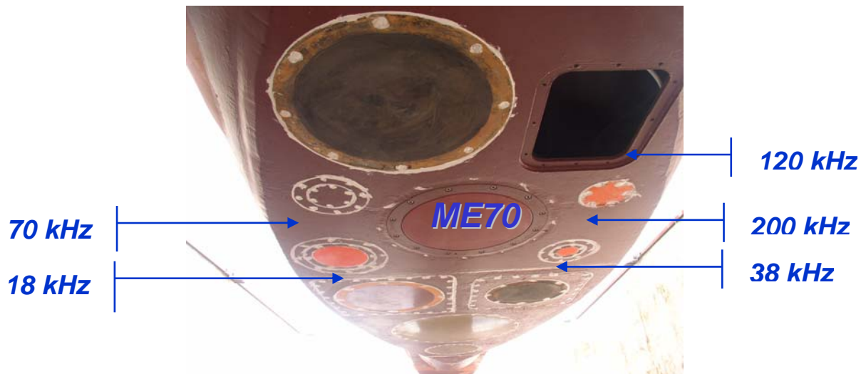
Figure 2. Relative locations of the EK60 and ME70 transducers on the hull of RV "Thalassa".
