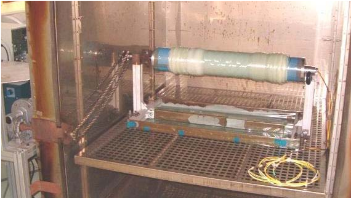
Figure 1. Cylinder installed on the turning mandrel inside the oven for the curing phase.
